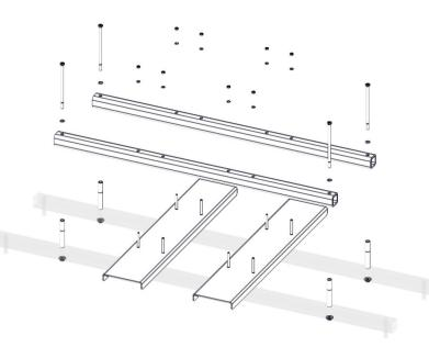
2. Place the angle lift lifting jigs on top of the forklift lifting bars in a perpendicular arrangement, aligning the screw holes of the angle lifting jigs and the lifting bars.
