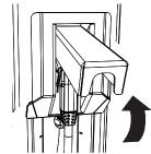
Open the station's door and pull out the connector.
