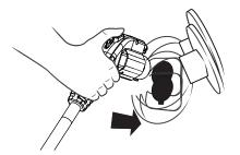
Plug the connector into your vehicle. Charging will start immediately.
