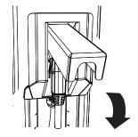
Once charging is complete, unplug the connector, replace it in its socket and close the door.
